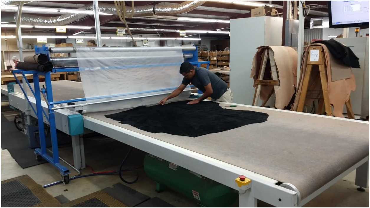
Computer controlled equipment cut saddle parts from hides.
